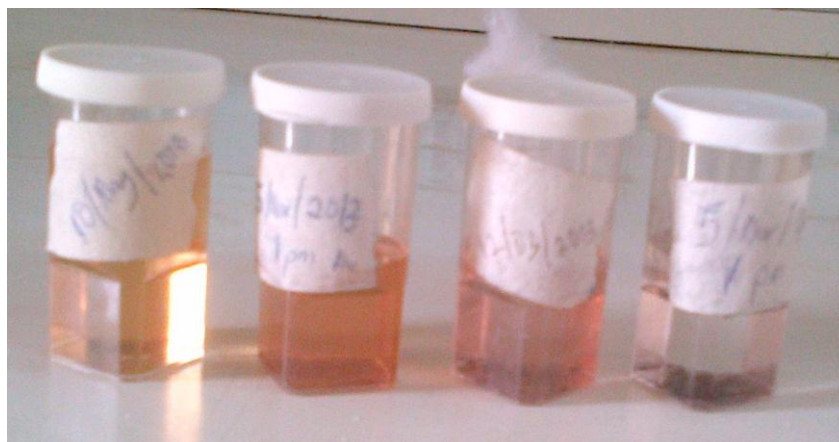
Figure 2 Colloidal silver in various stages of aggregation label a to d from left to right, a) clear yellow sol, b) dark yellow, c) violet, and d) grayish, as aggregation proceeds.
